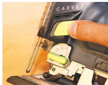
▲ Alternatively there are left and right sliders for inverted cutting operations
